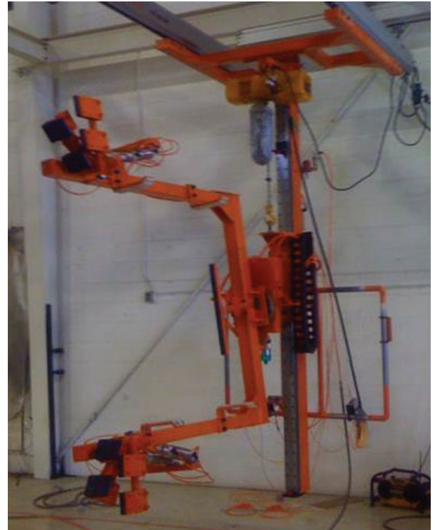
After this device lifts a watercraft, a motor rotates it 180 degrees
