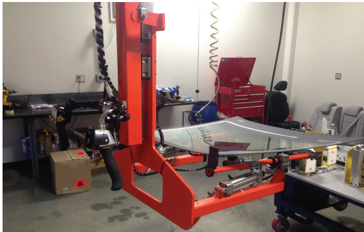
Cylinders tilt windshield 90 degrees into an upright position
