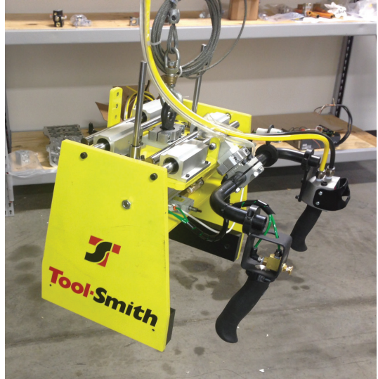
Clamping device actuated with pneumatic cylinders
