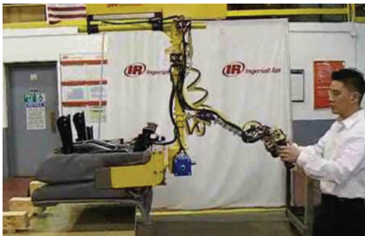
This device’s adjustable center of gravity allows it to pick up different sized parts
