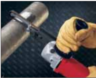
Strap polishing using contact arm 48-08-0290.
