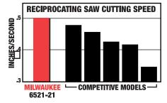
Source: Professional Service Industries, Inc. Note: Speed of cut in 1-1/8" particle board – 3 sheets clamped together
