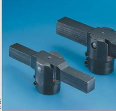
**▶** Clamp arms are used to transmit the force generated by the swing cylinder to the workpiece. The T-arm clamps two workpieces simultaneously with one swing cylinder. Enerpac recommend to use the pivoting T-arms with double-acting swing cylinders of the SU, SL, ST and SC-series.
