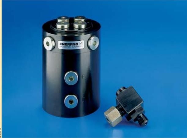
▶ Rotary couplers are specially designed unions to transfer pressurized fluid from a stationary supply line to a rotating device. Used for workholding or clamping device such as fixtures installed on rotating index tables.
