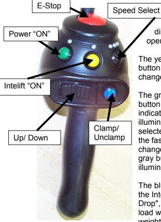
Select The green button turns power on to the controller, it will not disable the power nor will the Intelift operate until this button is pressed.
