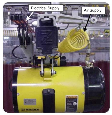
The preferred method of festooning is to install the electrification to one side of the runway and the pneumatic supply to the opposite side of the runway. This will prevent the two different supplies from entangling or abrading each other.
