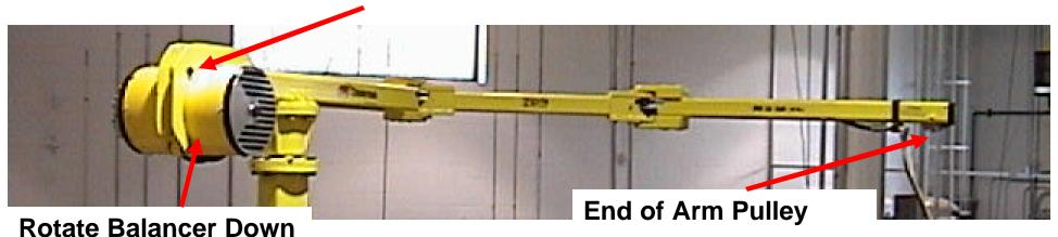
Cut Wire Rope at Balancer- Install new wire rope to reel- Butt Splice New Rope to Old Rope- At End of Arm Pulley Pull Old Wire Rope Out to Feed New Wire Rope through Pulleys
