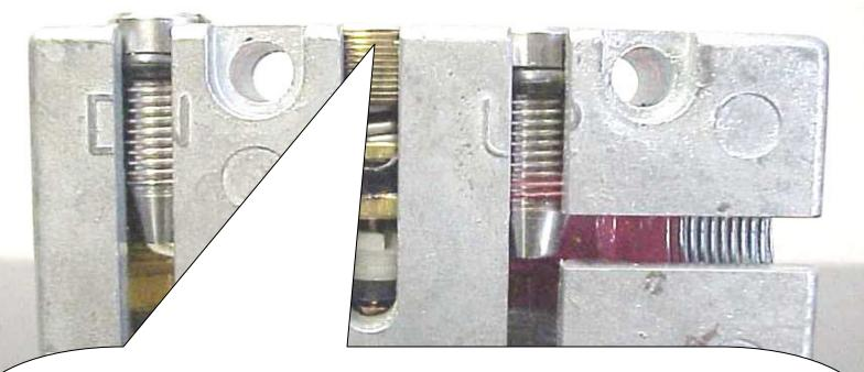
If the drifting continues after the Down line is pinched off check that the hook balance screw is flush with the top of the manifold block.
