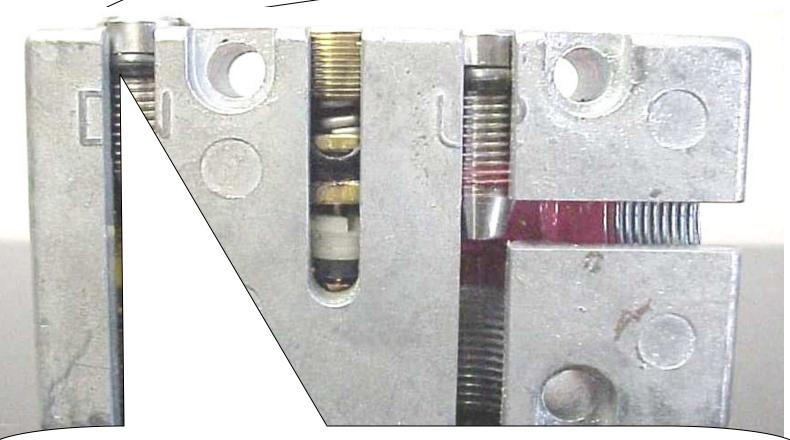
Spray leak check on the entire end cap if drifting continues.
