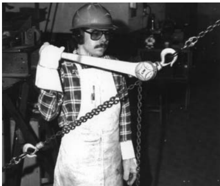
Figure 1. Pulling on an Angle
