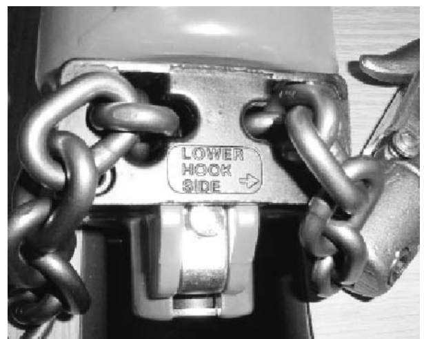
Figure 12. Chain Assembly - Hook End, 3/4 Ton
