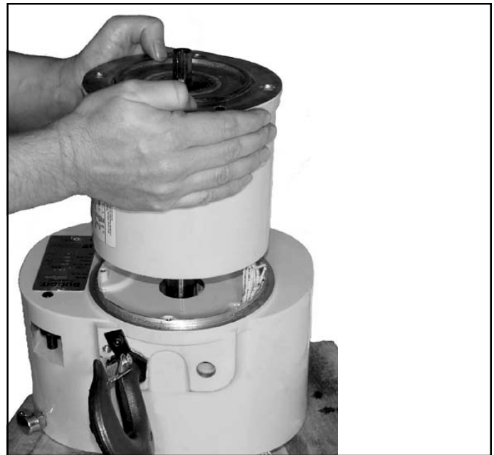
Figure 7-9. Removing Motor Assembly
