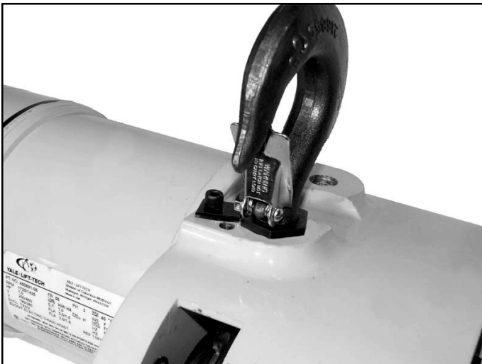
Figure 7-15. Removing Upper Hook and Hook Nut from Hoist Frame (1/4 thru 1 Ton Models)
