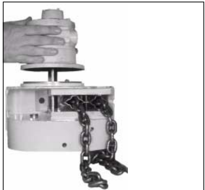
Figure 7-8. Removing Motor Assembly
