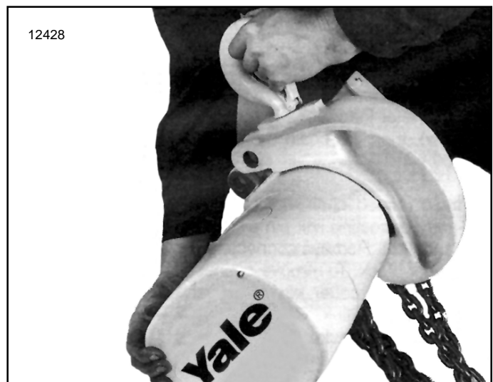
Figure 7-2. Removing 3 Ton Hanger Bracket from Hoist Frame
