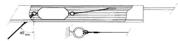
**IMPORTANT:** Thicker AK125, AK160 and AK200 conductors require a copper straightener Thread copper end though straightener before attaching pulling block. Straightener takes bend out of thick copper and assures easy pulling.
