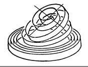
NOTE: It is recommended to replace all springs since unbroken springs of same age will likely need replacement very soon as well. Failure to do this will result in much more frequent maintenance.
