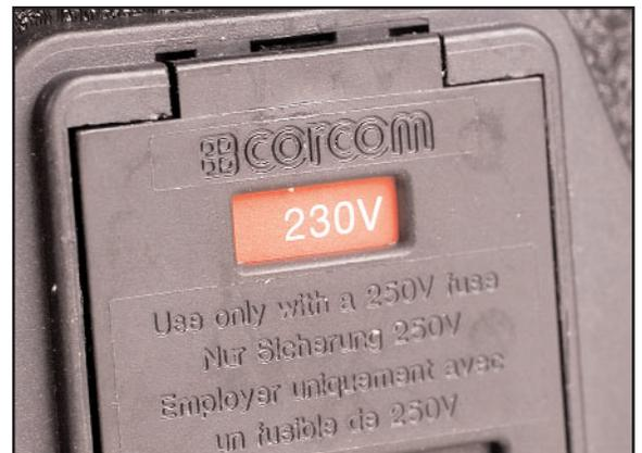
The PTV-FM is fused at 1 Amp for 115VAC. The PTV-FM is fused at 1 Amp for 230 VAC. The fuses are located on the sides of the voltage selector/fuse holder, as shown in the accompanying photograph.
