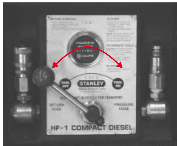
Figure 4. Control Panel to "ON" Position
