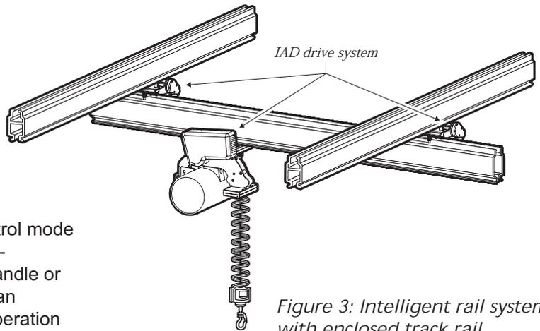
Figure 3: Intelligent rail system with enclosed track rail
