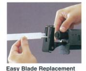
With Keyless blade clamping system, blade can be secured by just pushing the blade into the tool. And the blade can be easily removed by turning the holder collar.
