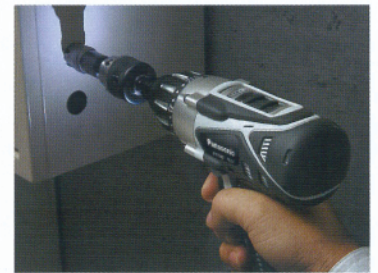
White LED light with condenser lens Even in the dark, areas for fastening screws can be clearly seen.
