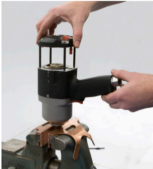
Figure 16.1 In preparation of disassembly, carefully clamp the anvil in a vise using copper jaws to protect the integrity of the anvil.
