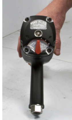
Figure 16.2 Turn the Reverse Lever to top dead center, or the twelve o'clock position before removing Back Cap Bolts.
