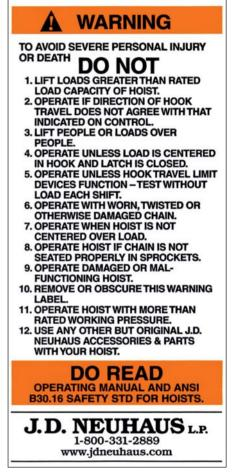
Warning tag attached to the control.
