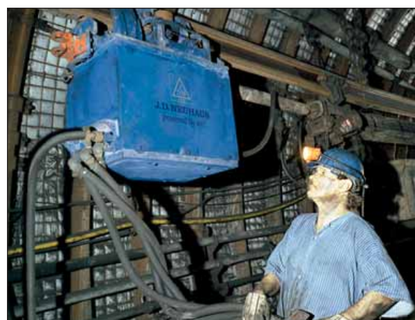
JDN Shunting Trolley SK 125 working underground.
