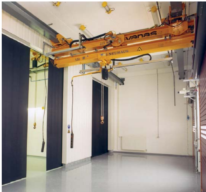
JDN Monorail Crane with wheel-away girder and trolley
