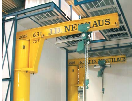
JDN Slewing Crane in a paint shop, carrying capacity 6.3t
