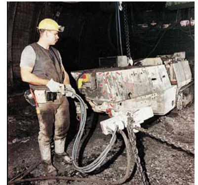
JDN air hoist B 612 rescuing a stuck loader
