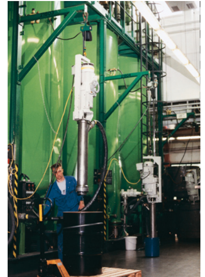
JDN air hoist mini handling a submersible pump in the chemical industry.
