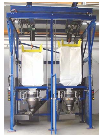
Big Bag Handling System with 2 JDN Air Hoists Profi 2 TI in Motor Trolley for operation in zone 1. The air supply is realised by a JDN Energy Chain. Most important in this case was that the Profis are suitable for oil-free operation.
