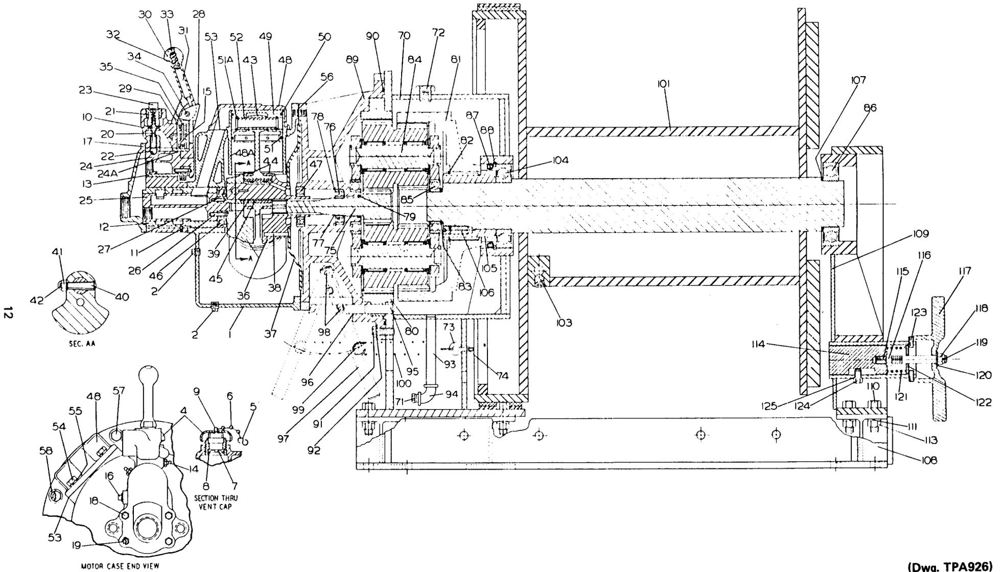
12UWB Winch with Manual Throttle, Manual Brake and Disengaging Clutch
