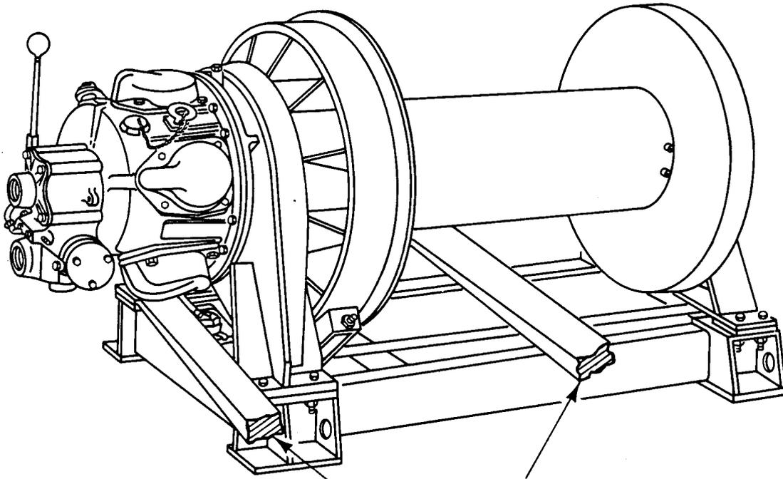
**Lifting Method Utilizing a Fork Lift
