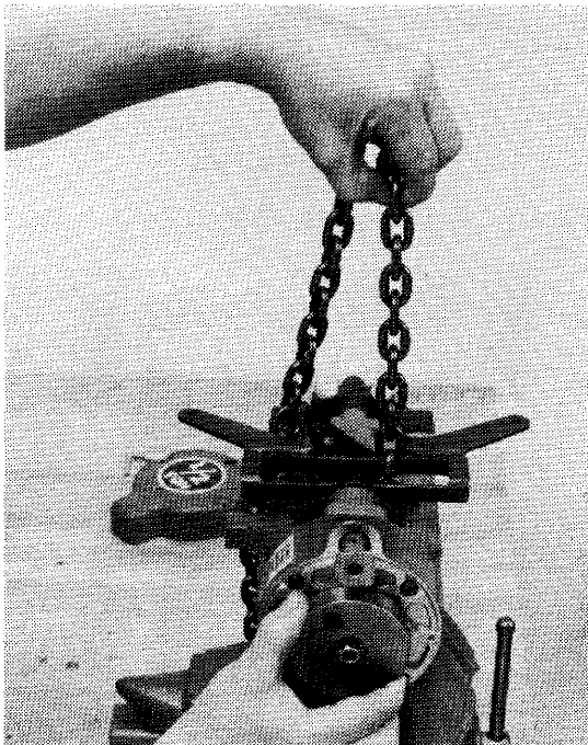
INSTALLING LOAD CHAIN
