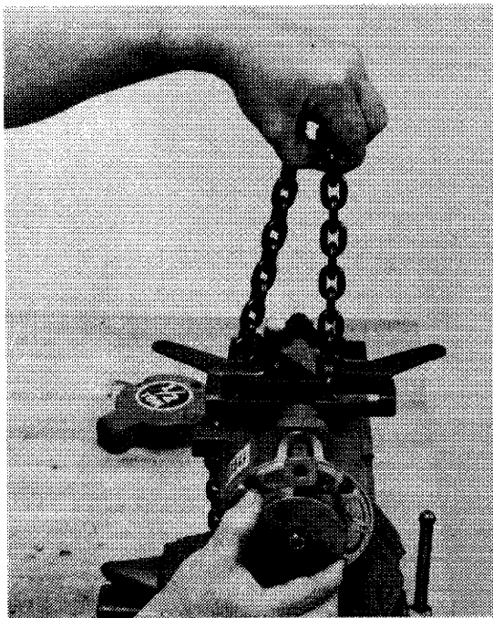
INSTALLING LOAD CHAIN
