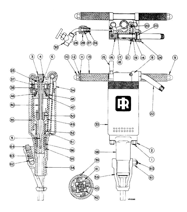
Figure 1. Jackhamer Model JH40 – Sectional Illustration (Yoke Type Steel Holder)
