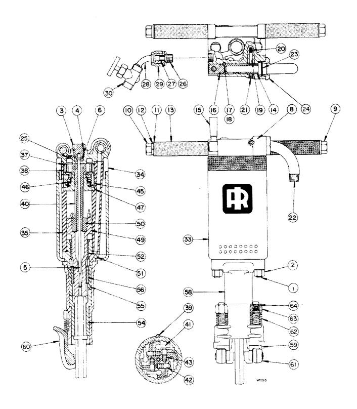
Figure 2. Jackhamer Model JH40 – Sectional Illustration (Yoke Type Steel Holder)
