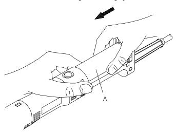
5. Push the Grip Latch downward to its original position to lock the adjustment into position. (Refer to Dwg.TPD1838)
