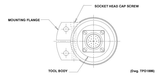
The Mounting Flange of all DC Electric Series DEMP Push-to-Start Torque Control Wrenches is attached to the Tool with a specific torque that is preset at the factory.
