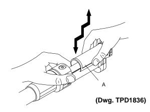
4. Slide the Grip forward onto the Handle until it butts against the Collar Assembly. (Refer to TPD1837).
