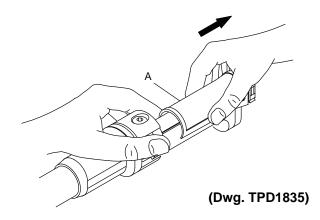
3. Raise or lower the Grip until the desired grooves inside the Grip align with the appropriate lugs on the Handle. (Refer to TPD1836).
