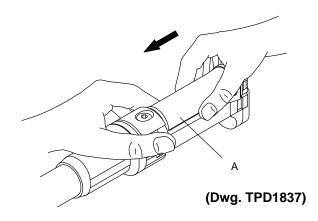
5. Push the Grip Latch downward to its original position to lock the adjustment into position. (Refer to TPD1838).
