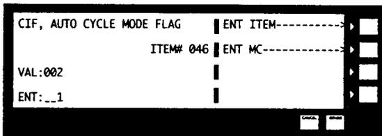
Computer accepts code 46 & brings up statement to assign the type of cycle mode. Computer is preprogrammed for mode 2 (default value).
