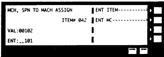
For the simplest set-up assign one spindle or tool to one machine by entering a value of 101 - tool 1 to machine 1. (See also Section 7.0 Two Spindle Operation)
