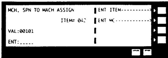
Code 42 statement allows you to assign different spindle configurations to a particular machine i.e., 1 spindle or tool to one machine - tool & machine are the same -for cases where you want to tighten two screws simultaneously with one fixtured control machine; the one machine has 2 tools.
