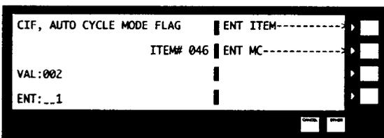
Reassign computer cycle start to mode 1, auto cycle start. Tool automatically is ready for next fastening cycle after the previous cycle completed.
