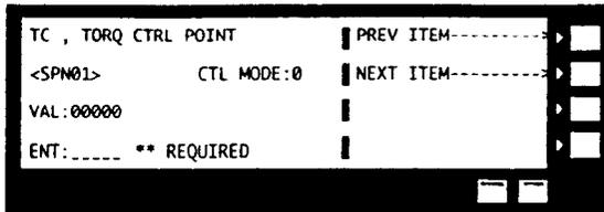
Brings up the torque control point statement which tells computer what you want the statistical data to be based on and also the torque value at which you want the tool to shut off.
