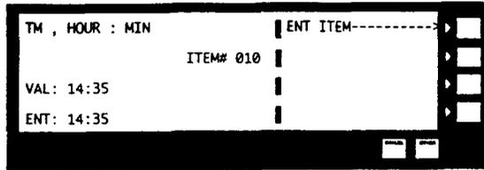
Brings up the time for hour and minutes on the 24 hour system to be programmed.
