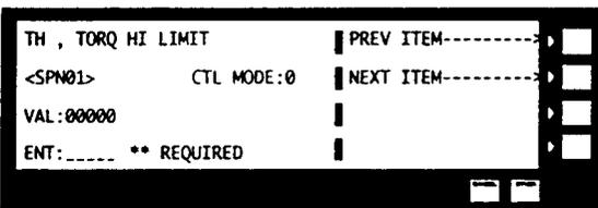
Brings up the torque high limit statement, when tool overtorques beyond this high limit (TH) error signal (red light goes on) and 'H' will appear after torque data.
