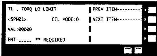
Brings up the torque low limit statement. When tool does not meet this low limit (TL) error signal (yellow lights) and 'L' will appear after torque data.
