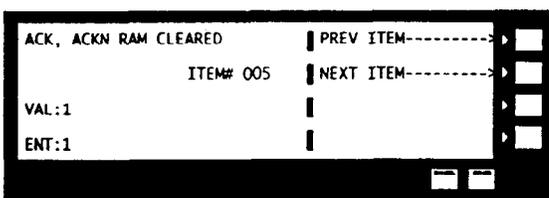
By programming a '1' into statement RAM clear ACK. We will reset the computer to be able to run tools and properly record data. More programming will be required however before you can run a tool. Computer is now reset.
