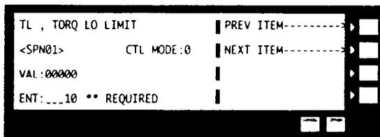
For this example let the lowest acceptable torque be 5 n-m below the desired torque. (TL = 15 - 5 = 10) Set TL at 10.
