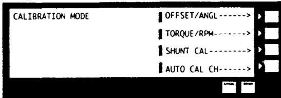
Calibration mode menu allows you to call up different functions required to properly adjust torque transducer
