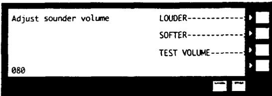
The user can increment and decrement and test the sound level by pressing the appropriate selection keys. Displayed in the lower left corner of the display is a relative sound level, which varies from 0 to 100H. The test will put up a message indicating when minimum or maximum level has been reached.
