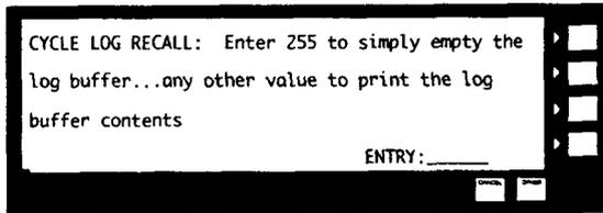
Pressing a key for an active report will provide the option to terminate its output ("\*\*\*" to the left of a report's function key means that it is already active). The display response will be:
