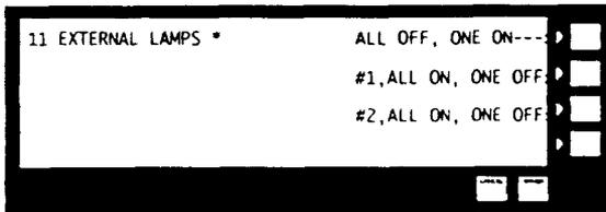
The test lights one lamp or AOK at a time for 0.5 seconds each. This sequence repeats itself until the operator terminated the test. All the external HI/LO and AOK lamps are turned off at this time. If the F2 or F3 key is pressed, the test will have all lamps initially on (for selected group) and turn lamps off one at a time. If F1 is pressed, the initial test is restored, i.e., all off initially, with lamps turned on one at a time.
