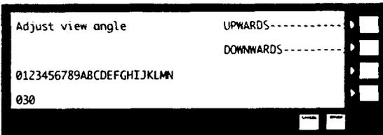
The user can adjust the view angle by pressing the appropriate selection keys. Displayed in the lower left corner of the display is a relative display angle value, which varies from 0 to 100H. The sequence 0-N is displayed for visual help in selecting the proper view angle.
