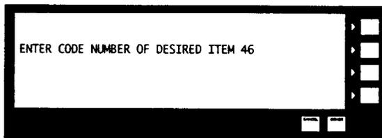
Select auto cycle start for spindle 1/machine 1. Use code #46 to do this.
