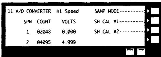
The test operates by, depending on input, closing or opening the shunt cal switch for the channels displayed. The display will show the A/D count and corresponding voltage for the spindle for display. Key F1 selects the origin of the A/D data, either the high speed sample routine or explicit read of the A/D converter. Keys F2 and F3 toggles the state of the shunt cal switch for spindle 1 and 2 respectively.
