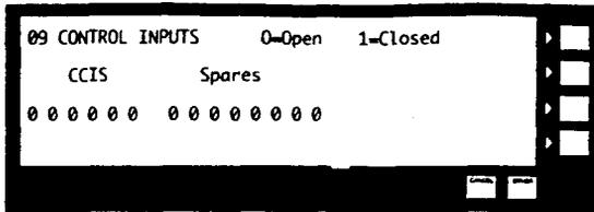
The display is used to indicate the state of the inputs. Each display bit (0 or 1) on the left corresponds to the state of one of the six optically coupled contact closure inputs (rightmost of the 6th contact closure is #1). The display bits on the right correspond to one of eight of the spare inputs. A contact closure on any input should produce a 1 indication on the display.
