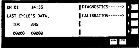
You are now ready to calibrate the tool i.e., adjust torque transducer to read proper torque.
