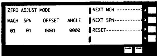
Ref. Fig. 4-5 - Number goes up and down as you slowly turn pot clockwise or counterclockwise respectively. Try to set as close to zero as possible.
