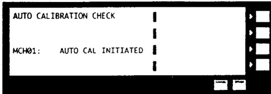
Brings up screen to have computer run through an automatic calibration check of transducer to verify if you calibrated properly. (if both yellow lights come on calibration is OK.) If not redo steps 66 to 74.
