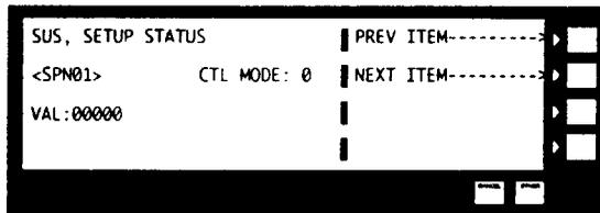
Skip all next parameter statements (TT, RTT, TDS) and stop when you see "SUS" (Set up status). This parameter is used to check if all data is entered properly.
