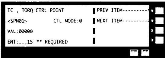
For our example let the desired target torque be 15 n-m. (set TC at 15)
