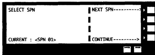
"NEXT SPN" key shuttles screen back and forth between spindle 1 & spindle 2.
