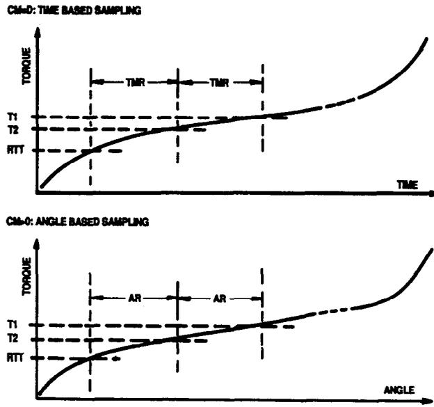
Figure 8-3. Run Down (Prevailing) Torque Monitoring
