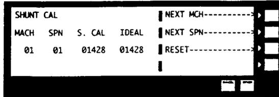
We must adjust the full scale value (Span) to 01428. The computer will automatically readjust to 1428 after each fastening cycle up to  $\pm 10\%$  ( $\pm 143$ ).
