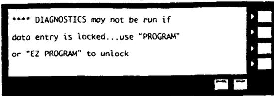
Pressing <CANCEL> will return the operator to the main display at which point he may select a "PROGRAM" function to access the unlocking mechanism. If the above condition does not inhibit entry to diagnostics, the program brings up the following additional warning message:
