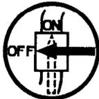
Turn off air supply and disconnect air supply hose before installing, removing or adjusting any accessory on this tool, or before performing any maintenance on this tool.
