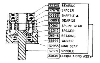
▲ INCLUDES NEEDLE BEARINGS, 15 PER SHAFT
