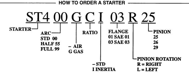
When ordering a Starter, refer to table below for correct pinion data.
