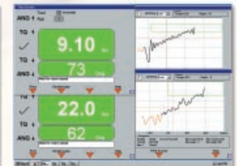
You can also launch multiple sessions to the same TME so you can monitor the Run Screen and the Oscilloscope at the same time.
